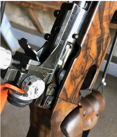
Opened action Suhl model 626-1 | Image credits (Hendrik Engelhardt, 2020, CC-BY)
